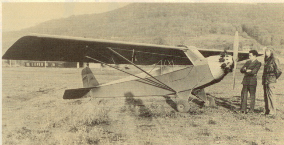
The prototype Taylor Cub with the French Salmson radial engine. Notice the drag wire from the wing to engine and the vane-type airspeed indicator on the right forward jury strut. Designer C. G. Taylor at left, test pilot Bud Havens at right. Photo courtesy of Gerald H. Balzer
