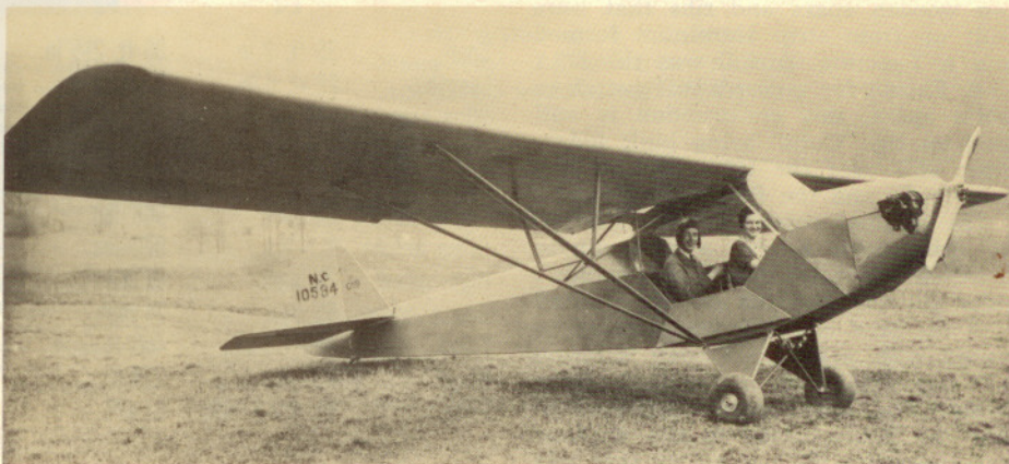
Production Taylor E-2 Cub with 37 hp Continental A-40 engine. Note the hinge-down door and the open cabin sides. The drag wires and external airspeed indicator of the prototype have been eliminated. Photo courtesy of Gerald H. Balzer
