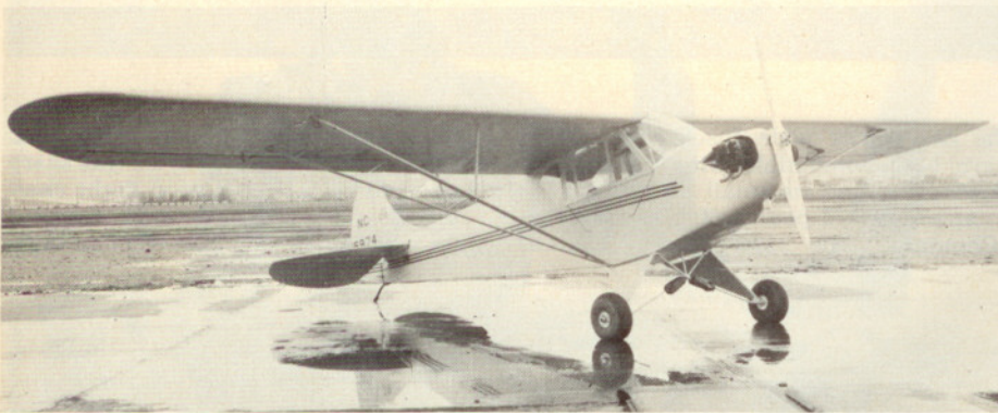
Taylor J-2 Cub, introduced in 1936, was essentially the same airframe as the E-2 Cub with new wingtip and tail shapes and the aft fuselage superstructure raised to the wing to make a bona fide cabin model.
